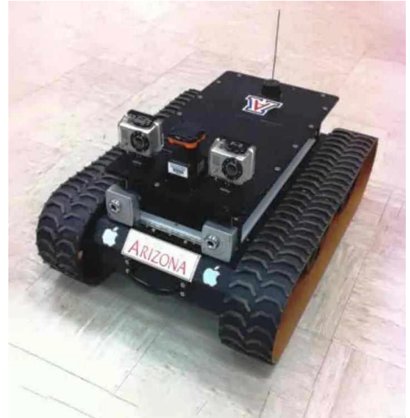
One of the experimental rovers used by Fink's team to test hardware and software related to autonomous exploration. This prototype is outfitted with cameras and other sensors for navigation. (Image: Wolfgang Fink/ University of Arizona)
